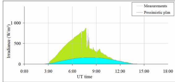
Figure 2: Insufficient use of available irradiance by a low linearization representing a theoretical overcast day
