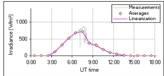
Figure 5: Algorithm for the linearization of the irradiance with null bias and minimum shifted irradiation
